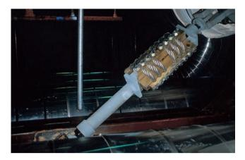
WEAR  $^{\text{TM}}$  (Wire Energy Absorbing Rope) pipe restraints are uniquely packaged wire rope isolators designed to protect structures from steady state vibration and restrain them from seismic and dynamic loads. The WEAR  $^{\text{TM}}$  pipe restraint will cushion, restrain and reduce energy into the structure through damping and will compensate for thermal expansion.
